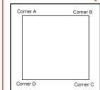
It is important to first insert graphic into each alternate corner, then to the sides of the frame. If this is not done, graphic will not fit into the frame correctly.
