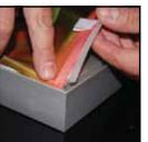
Insert corner A. Turn edge of graphic so silicon welt is perpendicular to face of graphic. Insert narrow side of welt with fabric to outside into the channel. Repeat for other side of this corner.
