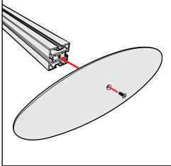
Base Plate & Extrusion Connection
